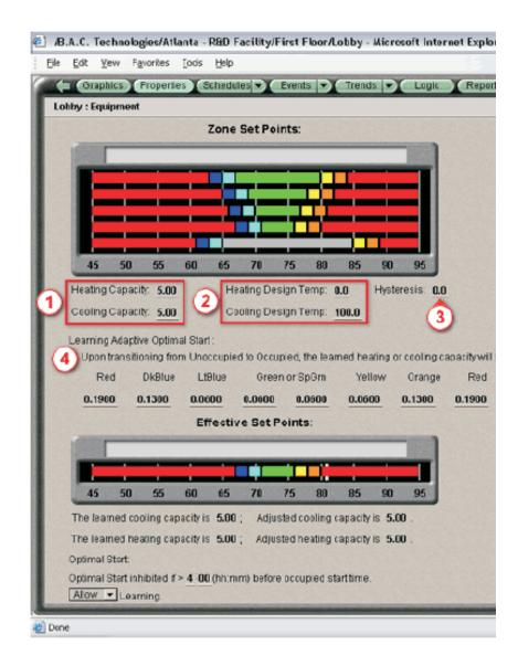
**4** The Zone Setpoint with Learning Adaptive Optimal Start microblocks can use the adjusted heating and cooling capacities to calculate current setpoints automatically.
